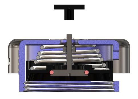
4) Remove the pallet assembly and pressure spring.
