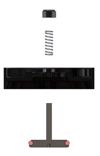
6) Remove the GF37000 vacuum o-ring.
