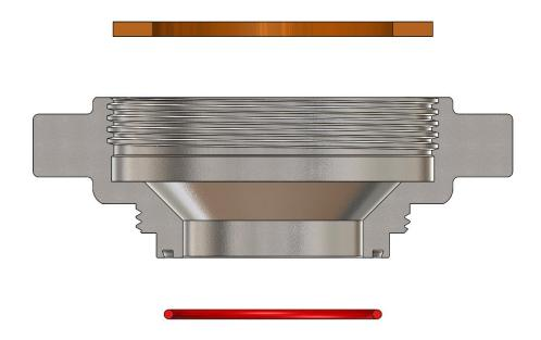
3) Insert flat head screwdriver into bottom of vacuum poppet to ensure it cannot turn. Unscrew and remove the GF39032 Vacuum Relief Button. **WARNING:** Device under pressure. Use caution when removing relief button and springs.
