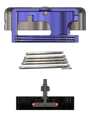
5) Unscrew the GF39010 VSK5V lock nut, remove the GF38020 vacuum spring, and remove the GF25002 vacuum poppet.
