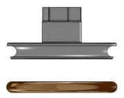
9) Remove piston rod and allow wiper to slide out of groove in assembly.
