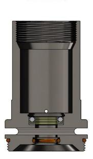
11) Remove and replace hydraulic seals and remaining O-rings.
