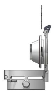
5) Remove the pressure/vacuum assembly from the housing and set the pressure spring aside.
