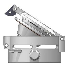
4) Carefully give the pressure/vacuum assembly (still attached to the flap) a 1/4 turn to release and remove the retaining clip. **Warning:** Use caution, as releasing the retaining clip will also release the compression force of the pressure spring.
