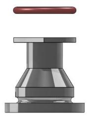
9) Remove and replace the body gasket from the lower housing, if required.
