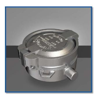
The dual-acting pallet of a Girard Vent/Fill IBC Cap relieves both pressure and vacuum, and sits securely within the vent body to avoid damage. Stainless steel construction and a choice of Teflon or Viton seals ensure compatibility with most any cargo. The device stands just 1 7/8" high (or 1" above the threaded flange), minimizing its exposure to collision.
