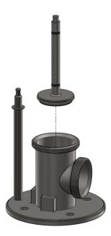
7. Finally, remove O-rings (GH60940) and main seal (GH60930) and replace.
