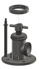
3. Screw handle back onto the threads until bottoming out.
