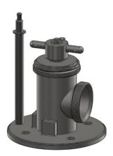
4. Remove cotter pin (GH60920) above the handle, then unscrew and remove the handle.
